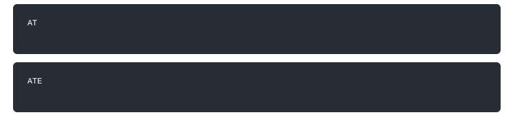
ATE will echo the commands you input to the module, which is useful for tracking the commands and troubleshooting.
