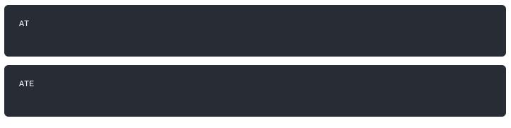
ATE will echo the commands you input to the module, which is useful for tracking the commands and troubleshooting.
